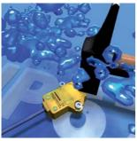
Made of high-quality plastic and IP67 rated, the housing provides high mechanical stability, protecting the sensor optimally against most chemicals and oils. The two-part build consisting of sensor and positioning element compensates lateral offsets of ≤ 3 mm and guarantees easy fitting and operation.
