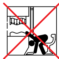
Reaching under from a crouched position
