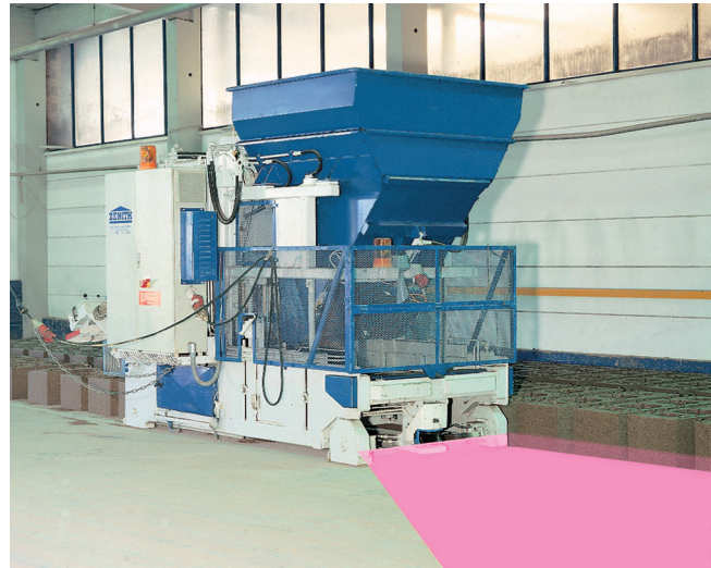
Protection of a mobile stone setting machine with SICK laser scanners
