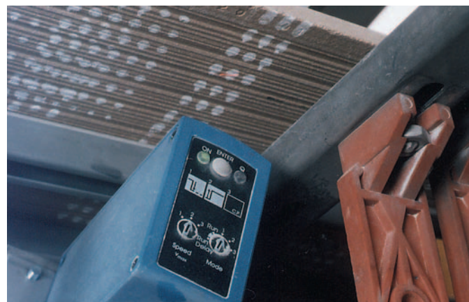
▲ Tiles checked to ensure that they are correctly positioned
