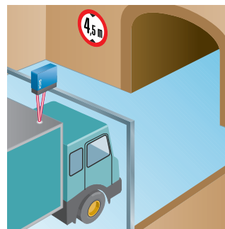
▼ Distance sensor: height control
