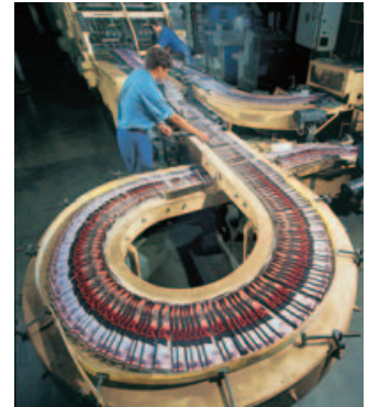
▼ Magazines being counted with DMH multifunction sensor
