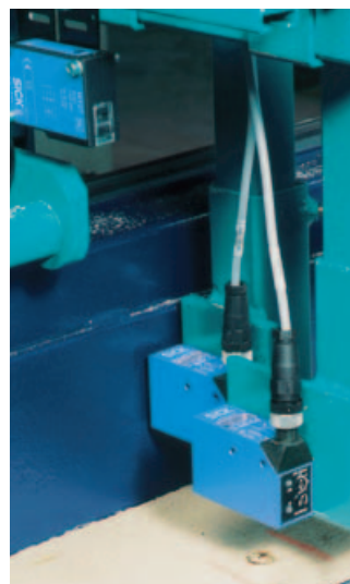
▲ Marks on planks are detected by luminescence scanners. Sawing is triggered.
