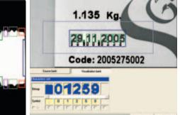
◄ Packaging and printing using OCR/OCV; The IVC-2D camera can not only check geometries, but simultaneously detect and read figures, letters, 2D codes and bar codes, e.g. sell-by dates for food or batch numbers on pharmaceutical packages. The camera system thus becomes a complete solution for inspecting a product's packaging and printing in a single pass.
