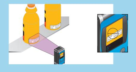
◀ With its robust and compact plastic housing and plastic front screen, the CVS4 is also particularly suitable for use in the food and beverage or pharmaceutical industries. And, thanks to IP 67 enclosure rating, it is particularly suitable for harsh industrial environments.
