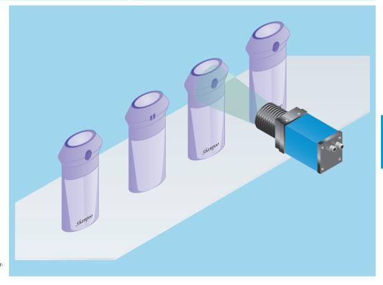
► Features such as grip mouldings, which reveal themselves by their reflective properties, can be used to control position.
