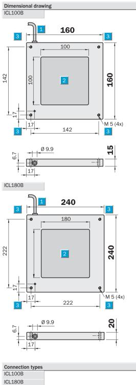
Cable with M12 plug, 8-pin Area illuminated
