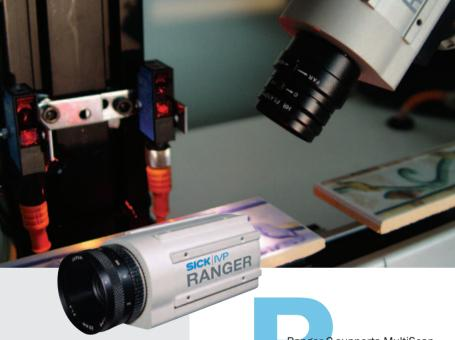
Ranger C supports MultiScan measurement – this means that the camera can acquire a number of properties (such as 3D, greyscale and scatter) of the measured object in the same scan.
