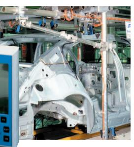
The ICS intelligent camera sensor integrates many functions and components into a single device and thus saves expenditure and space. Its compact housing contains all the components of a complete image processing system such as optics, object lighting, evaluation hardware and software.
