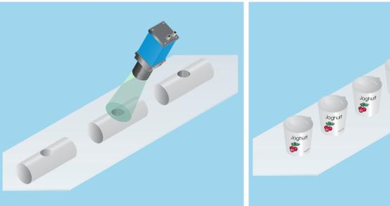
▲ Threads generate characteristic reflections which the AGD detects.
