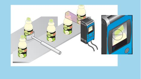
◄ With its robust and compact plastic housing and plastic front screen, the CVS3 is also particularly suitable for use in the food and beverage or pharmaceutical industries. And, thanks to IP 67 enclosure rating, it is particularly suitable for harsh industrial environments.
