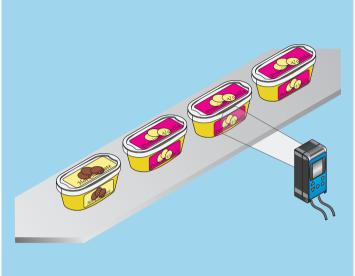
▲ Even parts with greatly varying appearance and position can be sorted by the CVS2, using their colour.
