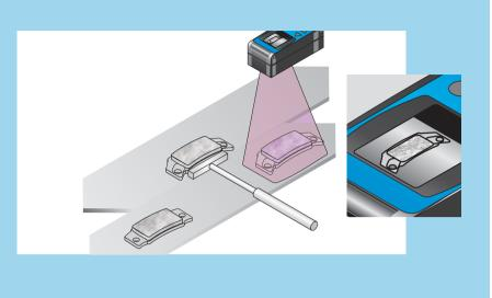
◄ The integrated memory can take teach-in data for up to 15 different objects; digital switching inputs permit external selection and, thus, fast and flexible product change-overs. During operation, all operational data required remains in view on the LCD display. Thus, the CVS3 combines all components of an image processing system in the smallest space.
