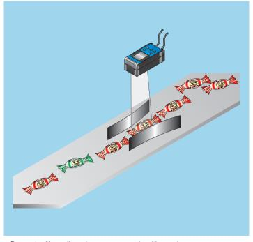
▼ The label is on – but is it the right one? The CVS1 Easy recognises incorrect labels by colour.
