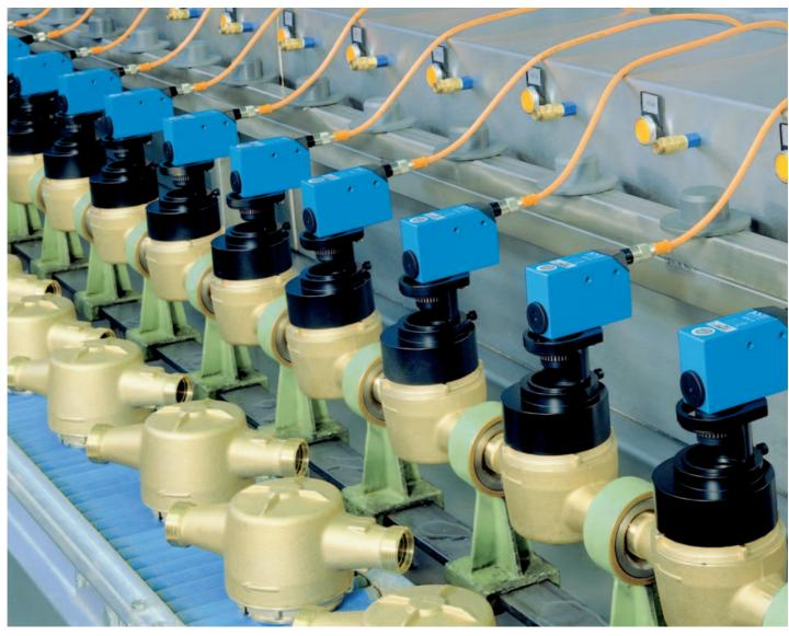
▲ KT contrast scanner in water meter manufacture
