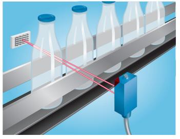
A newly developed system checks and continually adjusts the switching threshold electronically to adapt to the gradual accumulation of dirt, which would otherwise lead to a system failure.
