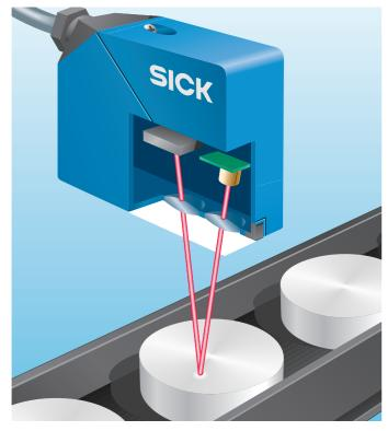
In the electronic method PSD elements (Position Sensitive Devices) are used. The emitted light beam is reflected by the object and hits the PSD receiver. Depending on the position of the reflected light beam, the incoming signal is recognised as being a background signal and electronically suppressed.
