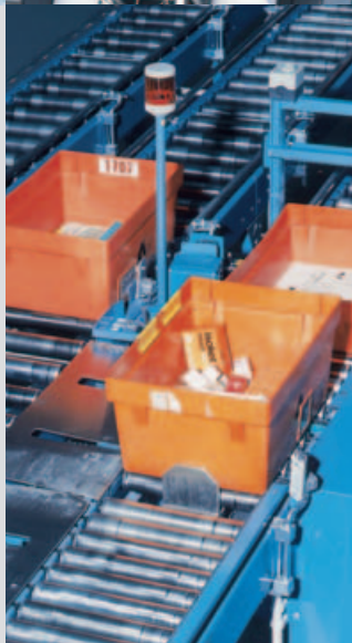
▲ SICK bar-code scanner systems control and monitor production and logistics processes.
