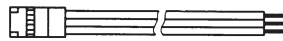
Connector with cable 0.5mm 2 Cable colors: OUT = green IN = brown GND = white
