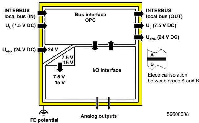
Figure 4 Electrical isolation of the individual function areas
