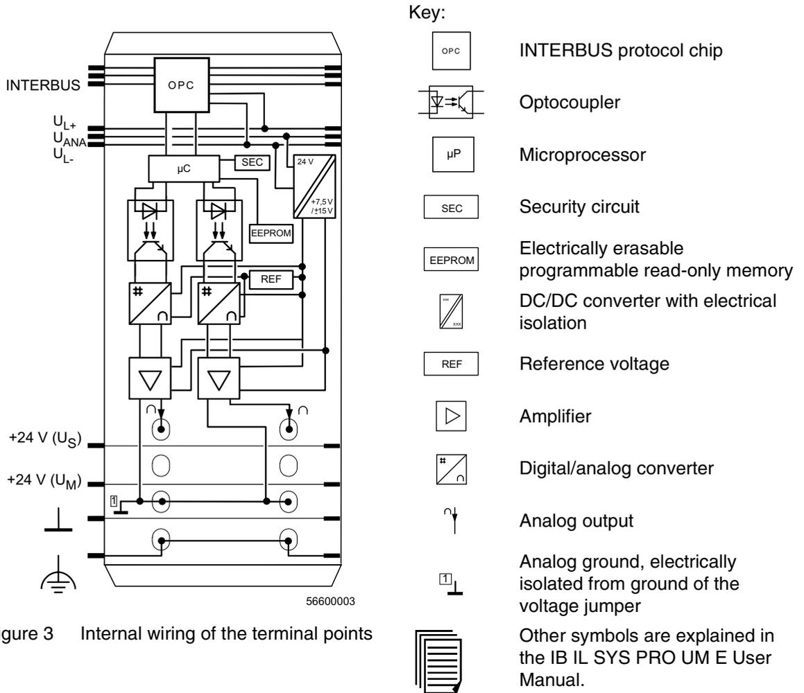
Figure 3 Internal wiring of the terminal points
