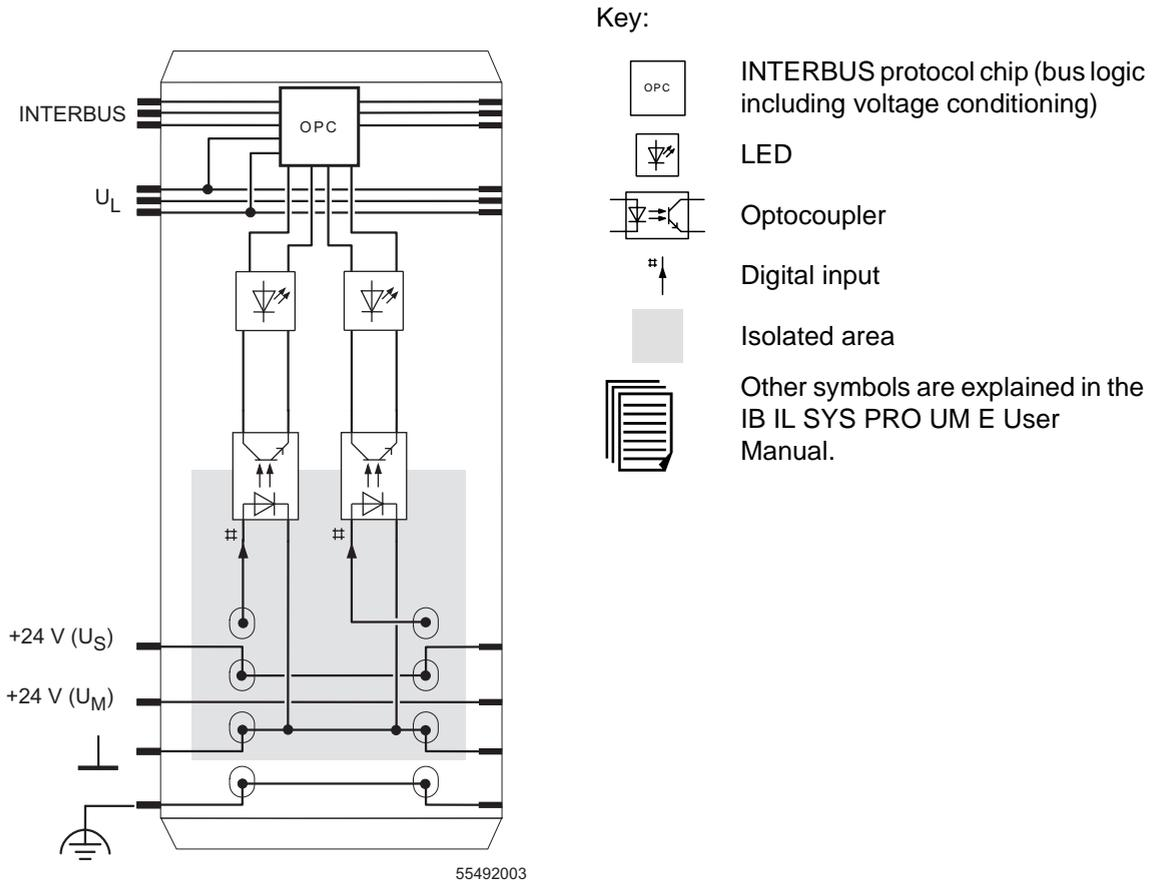
Figure 3 Internal wiring of the terminal points
