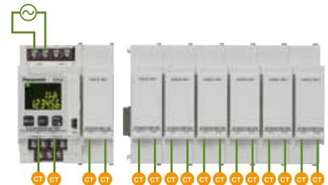
Add up to 7 expansion units! 8 measuring units total possible!
