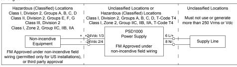
Non-incendive field wiring is not recognized by the Canadian Electrical Code, installation is permitted in the US only.
