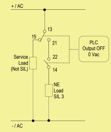
Contacts 13-21 and 14-22: the SiL 3 Safety Function is met when the relays are de-energized, contacts are open, NE load is de-energized.
