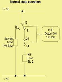
Contacts 13-21 and 14-22: in normal operation relays are energized, contacts are closed, NE load is energized.
