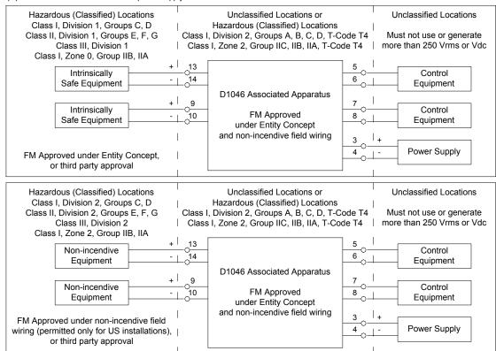
Non-incendive field wiring is not recognized by the Canadian Electrical Code, installation is permitted in the US only.
