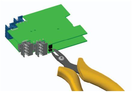
Cut both pins of the connector to open the wiring between the terminals, using a wire cutter
