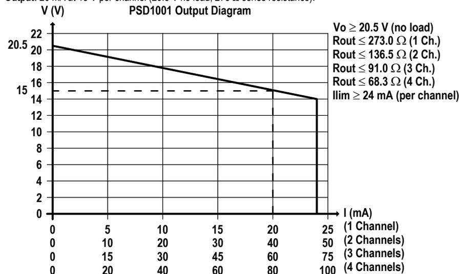
**Short circuit current:**  $\geq 24$  mA per channel (26 mA typical).
