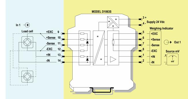
Up to 4 load cells 350  $\Omega$  in parallel Up to 6 load cells 450  $\Omega$  in parallel Up to 12 load cells 1000  $\Omega$  in parallel
