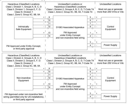
Non-incendive field wiring is not recognized by the Canadian Electrical Code, installation is permitted in the US only.
