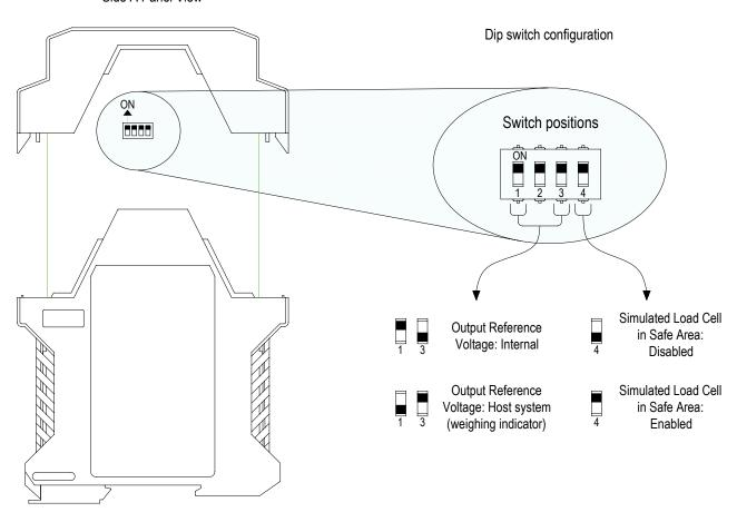
NOTE: to avoid damage of unit or weighing indicator always check reference voltage setting; to change the configuration always set before the dip switch from ON to OFF position prior from OFF to ON position the other:
