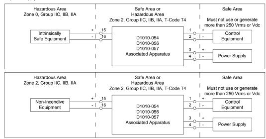
For installation of the unit in a Zone 2 location, the wiring between the control equipment and the D1010-05\* associated apparatus shall be accomplished via conduit connections or another acceptable Zone 2 wiring method.
