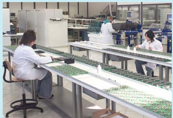
PTH component mounting after SMD line.
