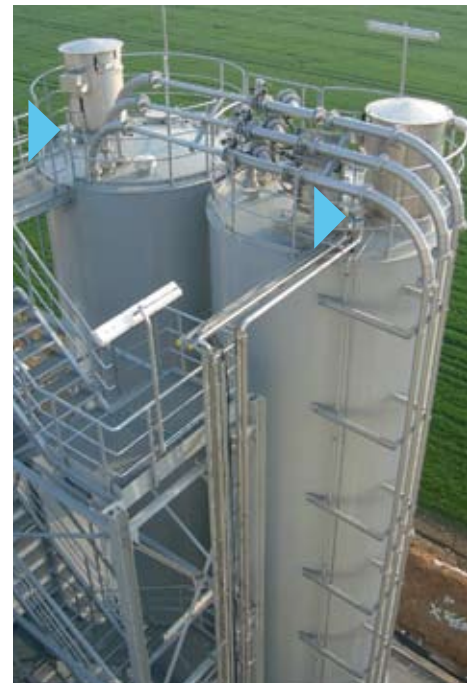
Residue silos, continuous level measurement of both residue silos by Levelflex M and Soliphant M
