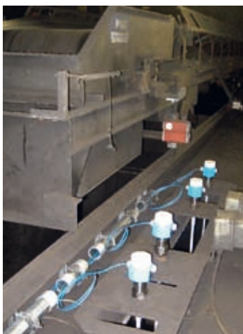
Solicap min/max detection in coal bunker
