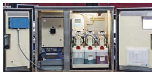
TopCal system in pH measurement for automatic cleaning and calibration
