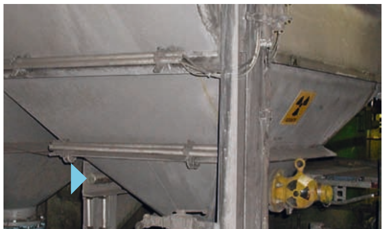
Gammapiilot for maximum limit detection in the electrostatic filter
