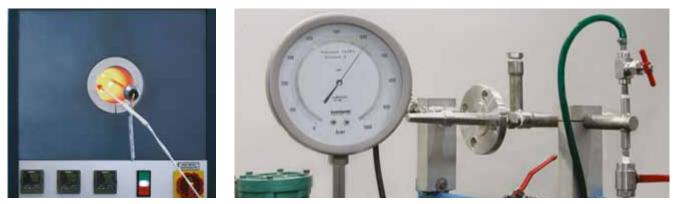
Performance test at 900 °C in a furnace and hydrostatic pressure test
