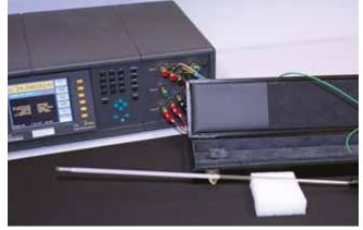
ITS90 calibrated, SPRT (Standard Platinum Resistance Thermometer) reference thermometer
