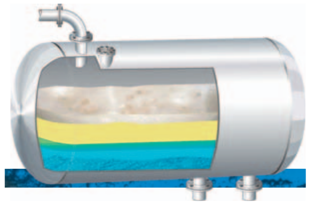
„Multilayer“ – Complex interfaces, for example in the crude oil extraction process
