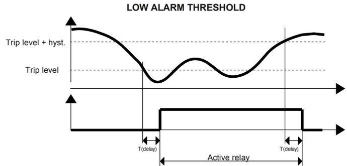
For the high alarm the relay goes on when the input signal is higher than the trip level and after the delay time. The relay goes off only when the input signal is lower than the trip level minus the hysteresis value or when reaches the minimum value of the input scale and after the delay time.
