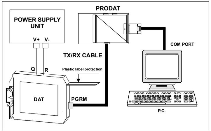
**Warning: during these operations the device must always be powered and the TX/RX cable always connected.**
