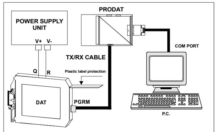
**Warning: during these operations the device must always be powered and the TX/RX cable always connected.**
