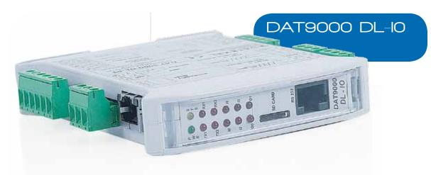
Intelligent Unit equipped with: n°1 interface RS-485 Modbus RTU Master, n°1 interface RS-485 Modbus RTU Slave, n°1 interface RS-232, n°1 interface Ethernet 10 Base-T Modbus TCP; N° 4 digital inputs; N° 2 SPDT relay outputs and micro SD card slot to memorize the data (Data Logger function). (AVAILABLE WITHIN DECEMBER 2010)
