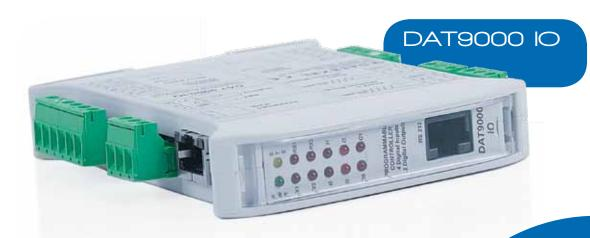
Intelligent Unit equipped with: n°1 interface RS-485 Modbus RTU Master, n°1 interface RS-485 Modbus RTU Slave, n°1 interface RS-232, n°1 interface Ethernet 10 Base-T Modbus TCP; N° 4 digital inputs and N° 2 SPDT relay outputs. (AVAILABLE)
