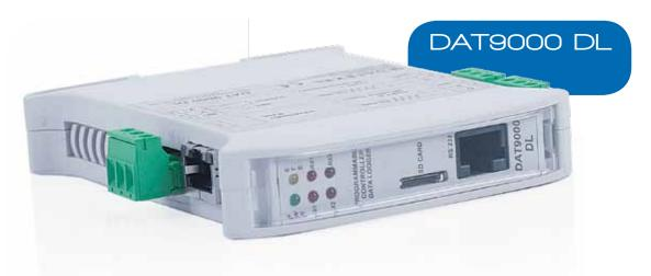
Intelligent Unit equipped with: n°1 interface RS-485 Modbus RTU Master, n°1 interface RS-485 Modbus RTU Slave, n°1 RS-232 interface, n°1 interface Ethernet 10 Base-T Modbus TCP and micro SD card slot to memorize the data (Data Logger function). (AVAILABLE WITHIN DECEMBER 2010)
