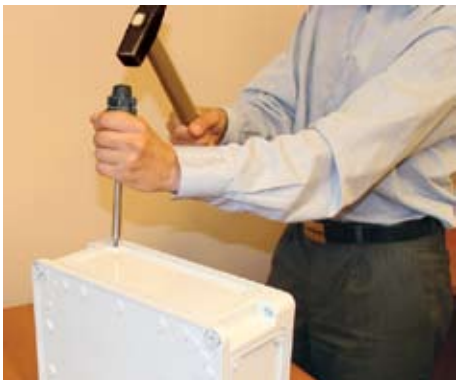
Move off the plastic from connection screw holes
