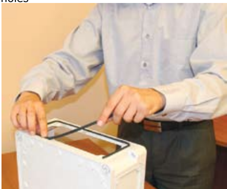
Install gasket to provide IP rating
