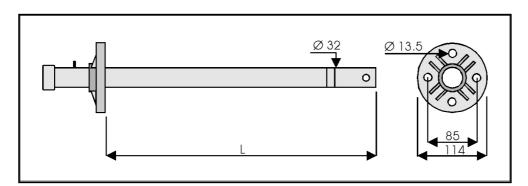
Fig.2 SI/32 IMMERSION PROBE OVERALL DIMENSIONS
