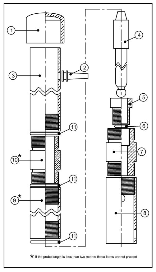
Fig.4 SI/32 ASSEMBLING SCHEME
