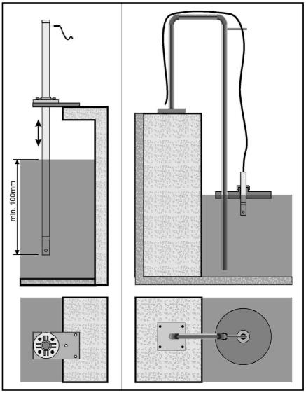
Fig.3 SI/32 PROBE TYPICAL SET UP
