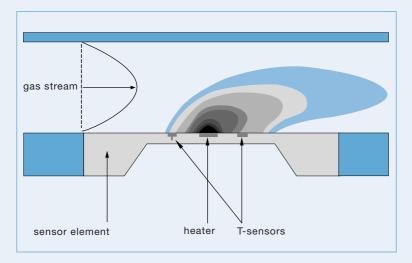
The actual flow rate is detected by a sensor operating according to a thermal principle which has the advantage of delivering the mass flow without any corrections for pressure or temperature being needed.
