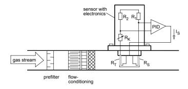
This sensor utilises the hot-film-anemometer principle in the so called Constant Temperature Anemometer mode. There are two resistances with precisely specified temperature coefficients directly in the gas stream as well as three resistances outside the gas stream interconnected to a bridae.
