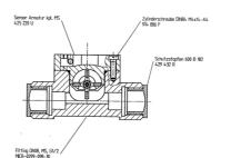
DN8 – stainless steel: Ident.: 439 410 Z Ordering key: SYST-S030-439410Z-SP229/99 Connection: NPT1/2 Length: 90 mm Machined: from a SS block 40 x 40 x 90 mm
