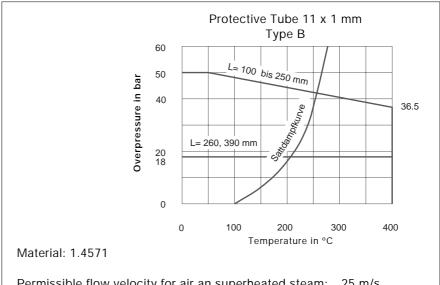
Permissible flow velocity for air an superheated steam: 25 m/s for water: 3 m/s
