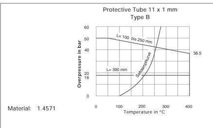
Permissible flow velocity for air and superheated steam: 25 m/s for water: 3 m/s
