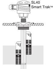
Up to four switches may be installed and adjusted to various depths on this in tank fitting called Smart Trak. Multiswitch installation is made both fast and simple.
