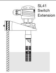
The switch extension fitting provides increased insertion depth for one switch. The optional side mount bracket may be used for installation to the tank's side wall.
