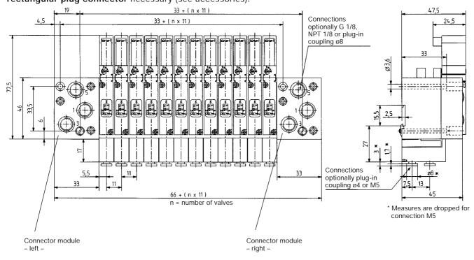
Block design with connector module on the right (1 supply port) and terminating module on the left; Block assembly with rectangular plug at the back (Version 1) and in front (Version 2) possible: rectangular plug connector necessary (see accessories)!
