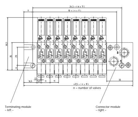
Specifications on design on a modular valve block, please see data sheet Customized Pneumatic Systems Solutions.
