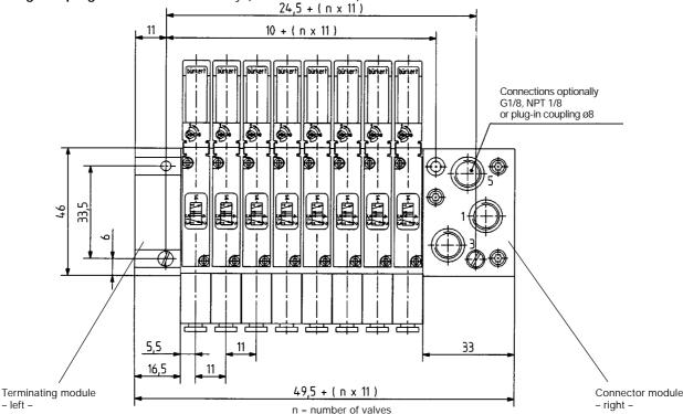
Specifications on design of a modular valve block, please see data sheet Customized Pneumatic Systems Solutions.
