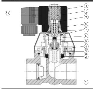
Valve body: Brass 2 Seat-seal: **NBR** 3 **PPS** Piston: 4 Gasket: **PTFE** 5 Spring: 1.4310 Plunger-seal: 6 **NBR** 7 O-rings: **NBR** 8 Plunger: 1.4105 9 Armature guide tube: 1.4301 10 1.4105 Stopper: 11 Coil Polyamide 12 Cable plug: Polyamide
