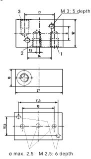
Multiple manifold for Burkert sub-base
