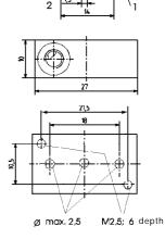
Type 6106 (3/2-Way) with side CNOMO manifold connection, circuit function C
