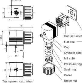
Flat seal Cylinder screw M3 x 30 Pressure ring Seal ring
