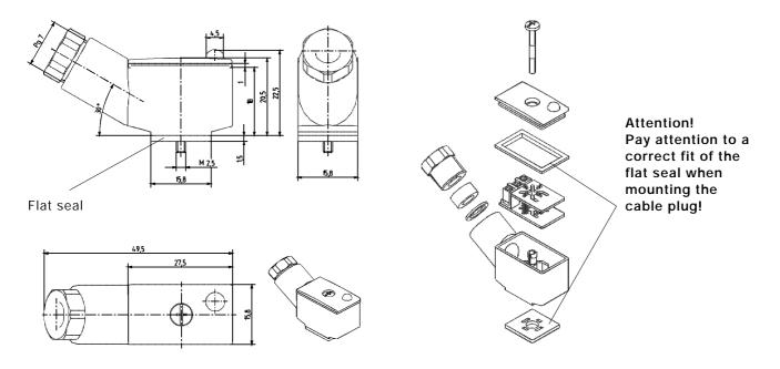
Cable plug type 2506 (pin assignment acc. DIN 43650, Form C)
