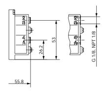
Version 4 Plug-in coupling legris ø 6 mm or threaded port G 1/8 (NPT 1/8 on request) in front, with one-way flow restrictor
