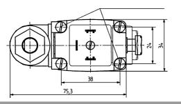
Valve with electrical feedback signaller Type 1060 (on request)
