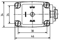
Valve with electrical feedback signaller Type 1060 (on request)
