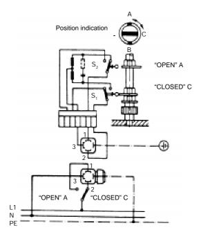
Version C with one potentiometer Version B with 2 additional limit switches
