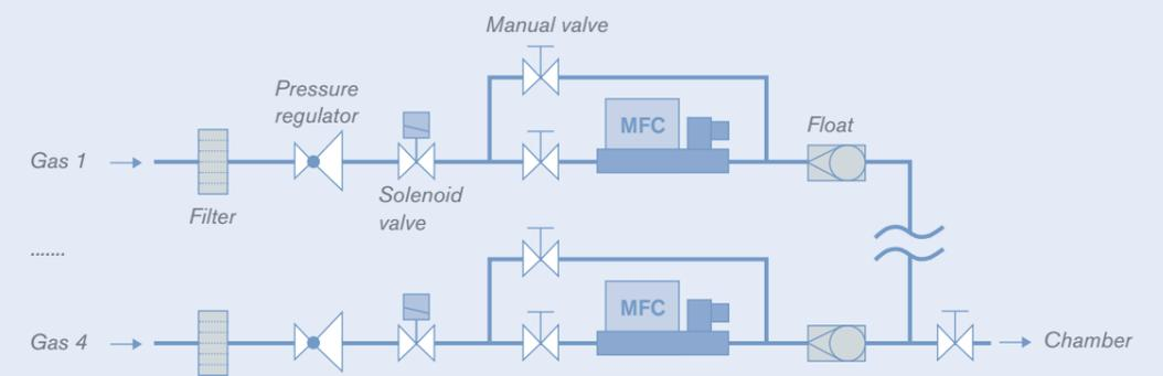
The MFCs provide defined atmospheres to guarantee reproducible processes. The atmosphere volume can range from a specific point on a weld seam to the chamber volume of a hardening furnace.
