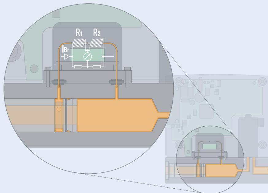
Functional schematic of the bypass measuring principle
