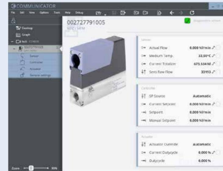
User interface of the Bürkert Communicator. The graphical programming interface (f(x)) is integrated into this software. The f(x) allows to program customized system control functions – e.g. for gas blending.
