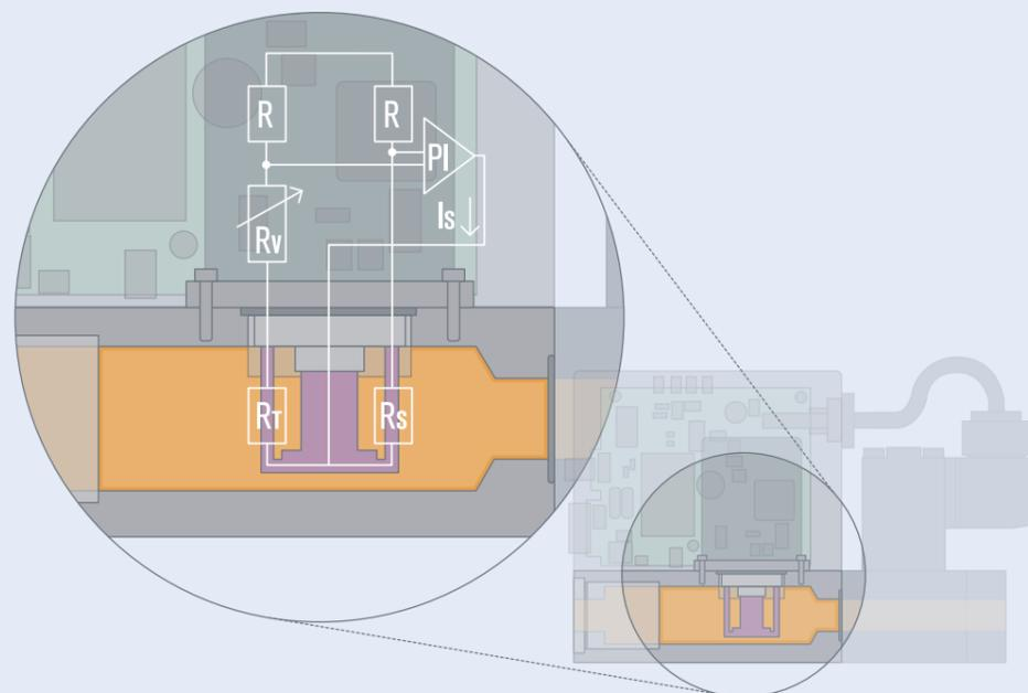
Functional schematic of Inline sensor
