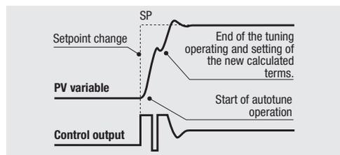
The **Natural frequency** method works best when the process variable is very near to the Setpoint. When activated, it causes a process oscillation around the Setpoint value.
