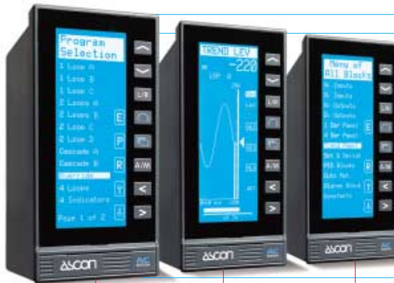
A single key stroke to select one of 12 preprogrammed control strategies stored in the instrument's library.
